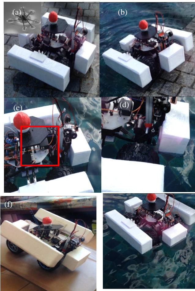
Fig. 6: UMT floats on the water surface mimicking a water spider gliding on the water surface (insets) (a) Ready to move on water surface, (b) Lifts down a pair of wings, (c) Moves on water surface, (d) UMT floats on water surface and releases the anchor into water surface and keeping UMT static at a position and (e) Retracts the anchor and continue moving, (f) UMT moves on a 20 cm height without the red object (ball) falling down.
